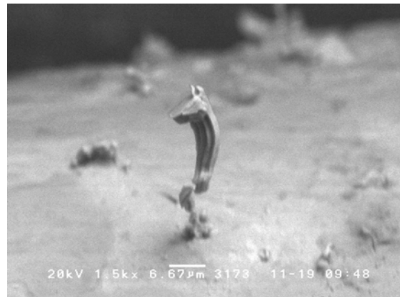
Figure 2 –SEM photograph of whisker formed on tin plated leads
