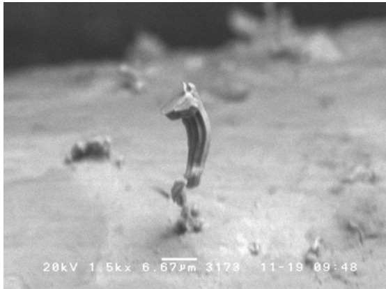
Figure 1 –SEM photograph of whisker formed on tin plated lead
